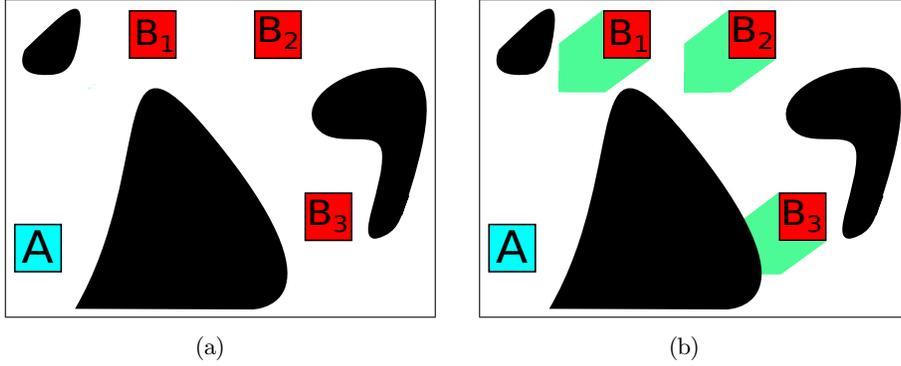
Fig. 1: (a) Basic PTAMP domain with one robot, three movable objects and obstacles. (b) Augmented PTAMP domain with shadows in green.
