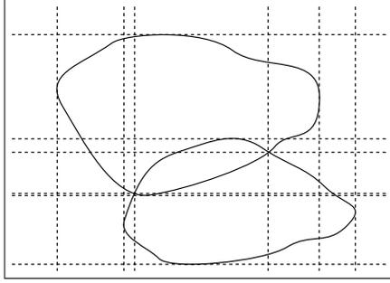
Fig. 3: Example FCAD decomposition. The resulting decomposition is the union of performing CAD with the decomposition orderings  $\{x, y\}$  and  $\{y, x\}$ .
