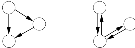
Figure 7: Two subassemblies that may be placed in a cell of the interference diagram.
