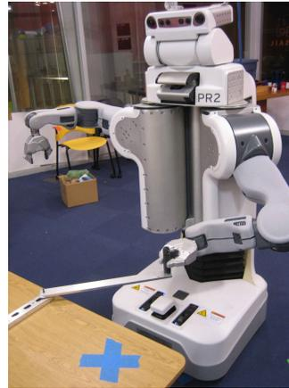
Fig. 1. Willow Garage PR2 robot manipulating revolute model
