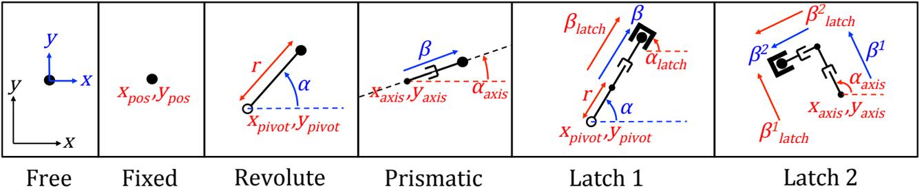
Fig. 2. Diagrams of the each of the 6 models considered. Fixed parameters are shown in red while variables are shown in blue. The large dot represents each mechanisms handle.
