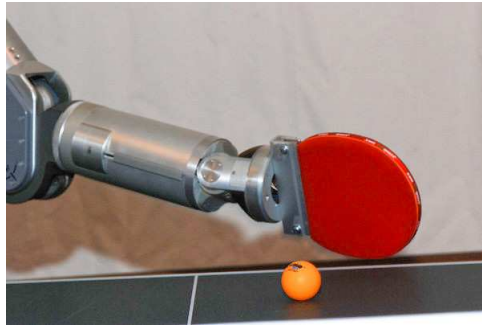
Fig. 1. Our ping pong robot uses a 7-dof Barrett WAM arm with a ping pong paddle rigidly attached at the wrist.
